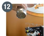
12. Check cans for leaks, flip upside down to ensure it is tightly sealed.
