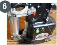
6. Using the adjusting handle, lift raising mechanisn to tighten can into machine.
