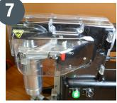
7. Close plastic guards to ensure safety during sealing process.
