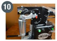
10. Lower raising mechanism using the adjusting handle.
