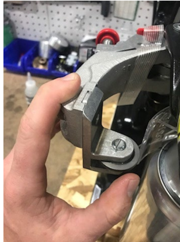
Spin roller by hand to drain lubrication between elbow and roller
