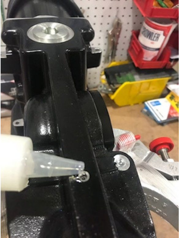
Drive Shaft Oil Point
